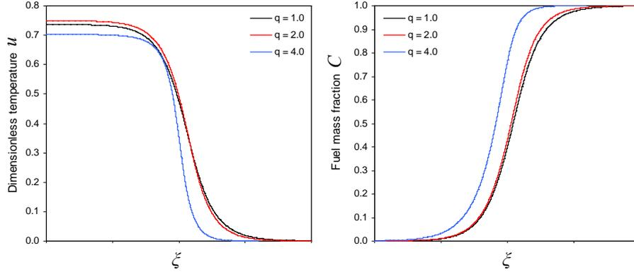
**Figure 1.** Combustion wave profiles arising in the competitive exothermic-endothermic scheme (2.1.1, 2.1.2) for three different values of the ratio of heats:  $q = 1.0, 2.0$  and  $4.0$ . The left panel shows profiles of the dimensionless temperature  $u_b$ , while the right panel shows the corresponding reactant mass fraction  $C$ . All of the profiles shown have dimensionless wave speed  $v = 0.355$ .
