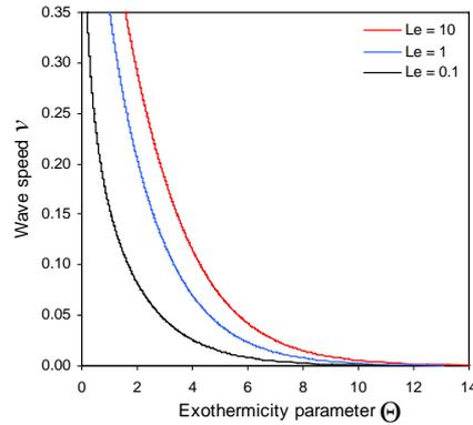
**Figure 2.** (a) Burnt temperature  $u_b$  and exothermicity parameter  $\Theta$  plotted against the ratio of heats  $q$  for combustion waves of constant speed  $v = 0.355$ . (b) Wave speed  $v$  plotted against the exothermicity parameter  $\Theta$  for different values of the Lewis number  $Le = 0.1, 1$  and  $10$ .
