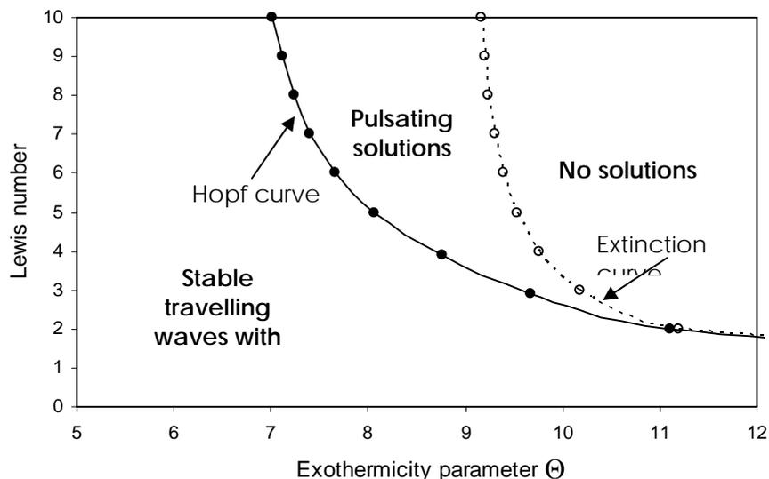
**Figure 5.** Stability diagram showing Hopf and extinction loci for  $f = 2, q = r = 1$ .
